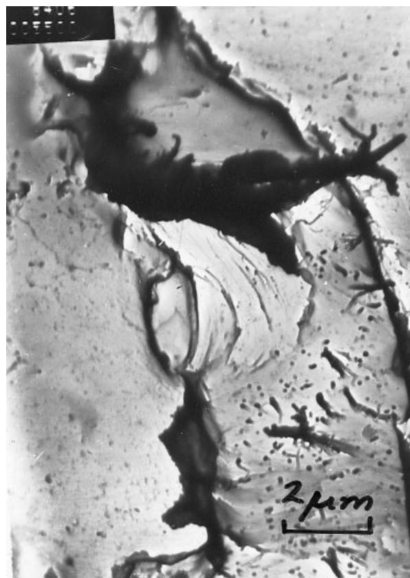
Figure 2 Electron photomicrograph of wood flour particles in the polymer matrix (NBR with 50 phr conifer wood flour).
